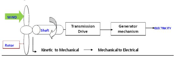
The above flow depicts the principle and mechanism of generating power from wind, Thereafter, the power generated by wind turbines is conditioned properly so as to feed the local grid as shown in below picture.
